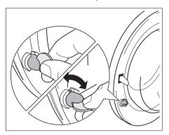
To disable this device and restore the possibility of closing the door, rotate the button counterclockwise until the groove is vertical.
